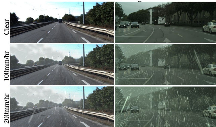
Physics-Based Rendering for Improving Robustness to Rain. Halder, Lalonde, and Charette, ICCV 2019
